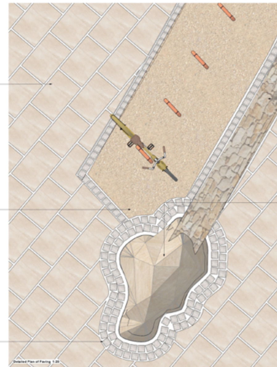
A key characteristic of my design is the paving details, using granite cobble setts to create a distinctive paving detail which is carried through the whole site
